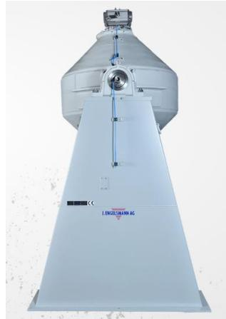
The mixing drum consists of a cylindrical middle section that ends with a conical end piece at the top and bottom. The connections for feeding and discharging the material to be mixed are located here. The mixing drum is mounted on shaft bearings, and the drive motor and control system are mounted on the side.
