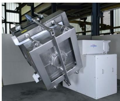
The JEL CM uses the principle of free-fall mixing to achieve homogeneous mixing of all ingredients – even with variable proportions and very small quantities. It is user-friendly, safe and works particularly gently.
